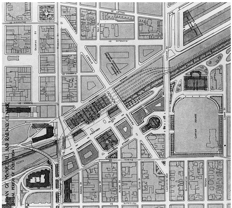
Figure 6. Plan of the proposed street and railway relocations to create a union railway station and municipal plaza adjacent to the Rideau Canal. Elgin Street is extended to create a diagonal view to the Parliament Buildings. (Source: FPC 1915, Drawing 6; drawing by office of E.H. Bennett; E.L. Cousins, consulting engineer.)
